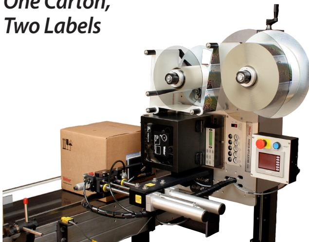
**The Model 5300 Twin-Tamp systems are specifically engineered to print a pair of labels and apply them to adjacent panels of cartons in a single operation.**
